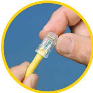
STEP 7 Slide assembly into plug body.
