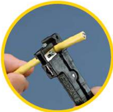
STEP 1 Strip and remove 4" of jacket.
